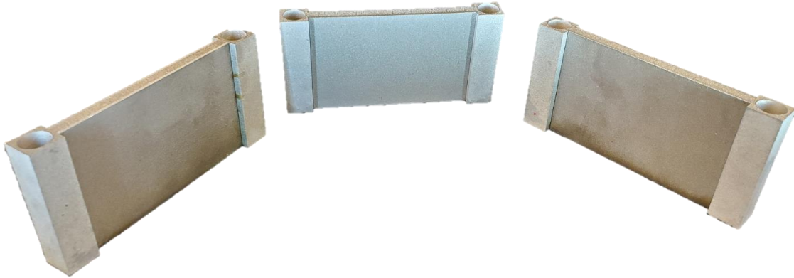
Figure 76. A set of novel CALPEs fabricated with stainless steel 3D-printing to maximize capillary height and heat removal capacity.
