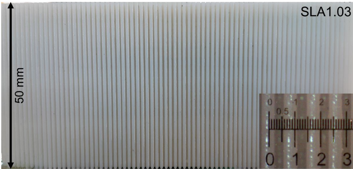
Figure 30. Micro-grooves made by stereolithography (SLA1.03) were used for the capillary rise measurement. The inset shows a micro-groove thickness of 500 \mu\text{m} and a micro-groove width of 400 \mu\text{m} . Micro-groove depth is 1 mm. Table 4 lists the sample details.
